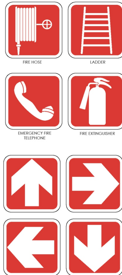
Exhibit 27: FIRE FIGHTING SIGNAGES
